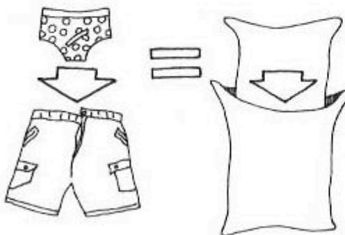
The lowest couple can be 'double bagged' for extra protection. Thus the gravel or the trench surface cannot tear the bag and spillages are avoided.
