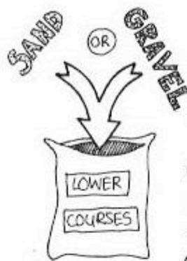
The first few courses of earthbags (all the 'below ground level' courses) should be filled with sand or gravel to prevent water wicking into the walls
