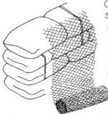
Chicken mesh is stretched over the earthbag wall. This provides a rough base for the plaster to hold on to.
