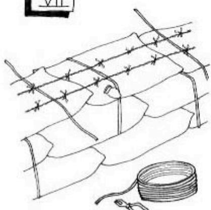
Binding wire/straps are placed on alternate bags to tie the course!
