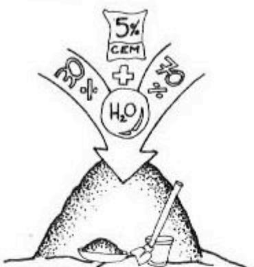
Water is added to the cement stabilised earth mix
