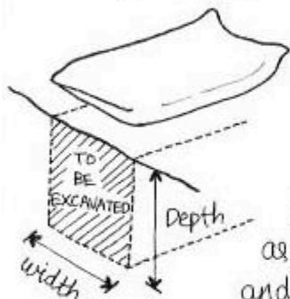
The width of the foundation trench should be slightly larger than the bay width.
